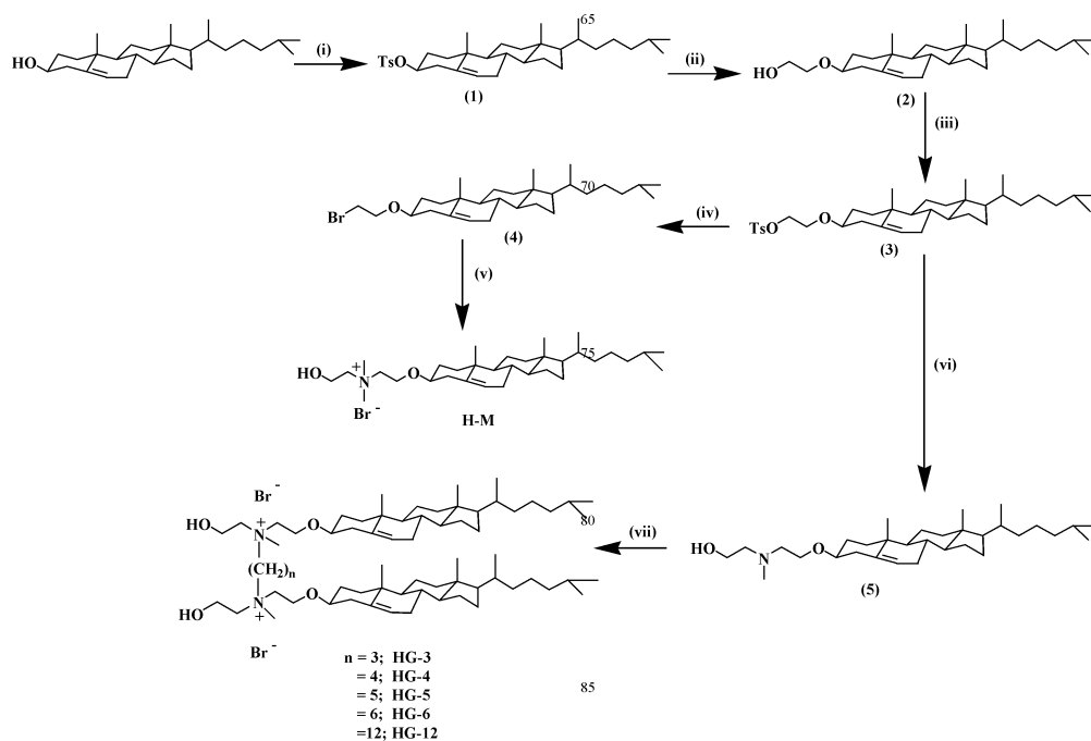
Scheme 1 Reaction conditions. (i) p -TsCl, Py, CHCl 3 , DMAP, 92.8%; (ii) Ethylene glycol, dioxane, reflux, 85%; (iii) p -TsCl, Py, CHCl 3 , 90%; (iv) LiBr, DMF, N 2 atm., reflux, 95%; (v) N,N -dimethylethanolamine, EtOH, screw-top pressure tube, 81%; (vi) N -methylethanolamine, CH 3 CN, reflux, 97%; (vii) Br-(CH 2 ) n -Br, EtOH, screw-top pressure tube, 70 °C, 40–50%.
